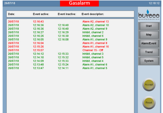
Event log with alarms, actuals (red), faults (green) incl. date and time
